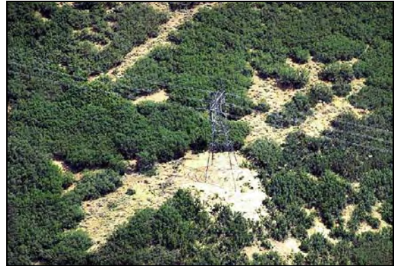
Using existing openings, lines, and shapes in the landscape can help reduce visual impacts.
